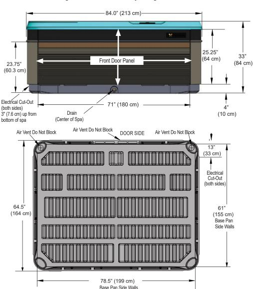
**NOTE: WATKINS WELLNESS** recommends that the **RAVELLO** be installed on a minimum 4" (10 cm) thick reinforced concrete pad or structurally sound deck able to support the "dead weight" found in the spa specification chart. **WARNING:** The **RAVELLO** must not be shimmed in any manner.
