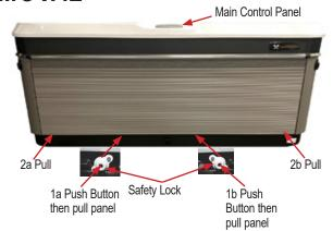
Pull (with slight force) on bottom left corner until panel un-clips followed by the right corner until panel un-clips.
