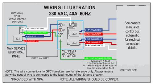
**WARNING!** The exact physical location of the terminals on the GFCI breaker will vary between manufacturers. Connecting the hot wire to the neutral terminal will cause irreversible damage to the control box.
