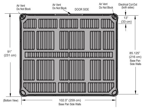
NOTE: **WATKINS WELLNESS** requires that the **CANTABRIA** be installed on a minimum 4" (10 cm) thick reinforced concrete pad or structurally sound deck able to support the "dead weight" found in the spa specification chart.
