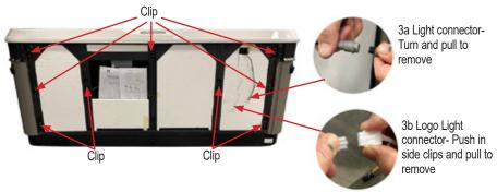
3 Pull bottom door panel away (using both hands spaced shoulder length apart) from each side of the spa center, this may require a slight amount of force because of the upper clips until they all un-clip. Lower panel to ground. Disconnect both the logo light and front light wires from door panel, then remove door panel from spa area and set in a cool shaded place. Remove foam to access.
