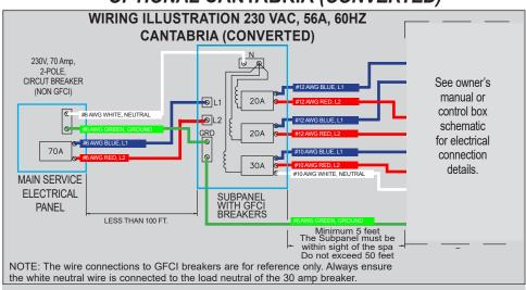
NOTE: ALL WIRING SHOULD BE COPPER.
